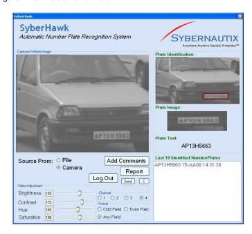
Once the vehicle was captured by the camera, the frame is automatically sent for the recognition. After recognition, red line appeared around the plate location and the registration number was displayed along with the time of identification (see above image).
